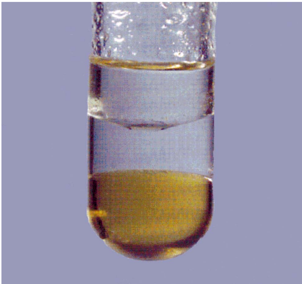
Figure 1. A triphasic mixture of [\text{bmim}]_2[\text{PdCl}_4] and \text{P}(o\text{-tol})_3 in [\text{bmim}][\text{PF}_6] (lower layer), water (middle layer), and cyclohexane (top layer).
